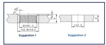
Recommended install torque 0.7-1.0Nm, do not exceed 2.5Nm
